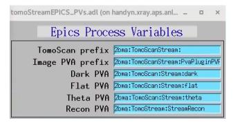
to set the TomoScan prefix and the PVAccess names provided by tomoScan for projection (Image), dark and flat image broadcast. Here also set the Recon PVAccess name where the streaming reconstruction will served. Use the Recon
